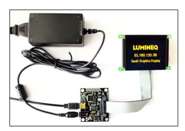
The USB13700 Demo Kit offers a quick and easy means to demonstrate the capabilities of small graphics Lumineq<sup>®</sup> TFEL displays with a PC.
